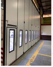
The Osprey door is horizontally moving, operated by a variable speed drive unit which slides and folds all ten leaves behind the reveal, leaving the full 9.5metre width opening clear for vehicle access. In the closed position, the door is completely flat across the opening. Soft compound EPDM weather seals to all edges eliminate water, air and dust ingress, and a stainless steel bottom
